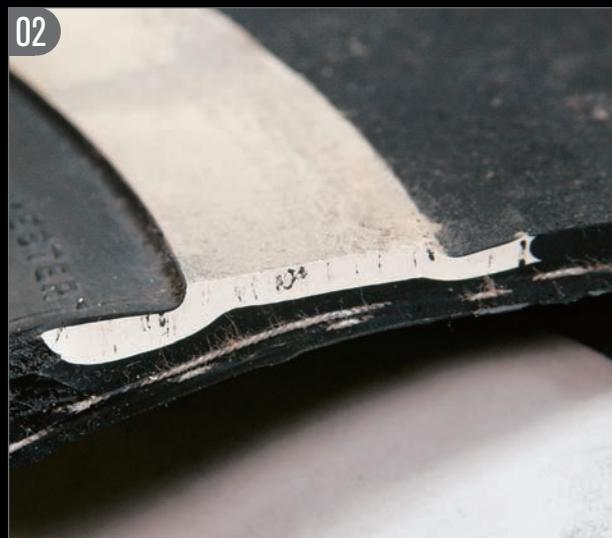
Using a junk tire, we cut through the sidewall to show just how wide the ring of naturally white rubber is on the average whitewall tire. As you can see, a very thin layer of black rubber covers much of the available white rubber. The cutaway view shows that grinding back the thin layer of black rubber will have essentially no effect on the strength of the tire's sidewall.
