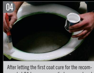
After letting the first coat cure for the recommended 24 hours, we applied a second and third coat in 24-hour increments as the manufacturer suggested.
