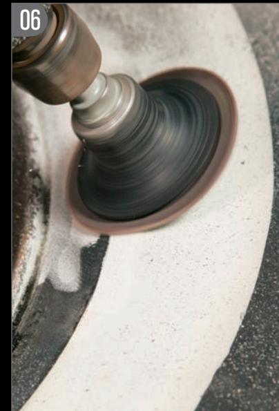
To remove the black rubber from the inside radius, we used a smaller pneumatic 3-inch right-angle die-grinder.
