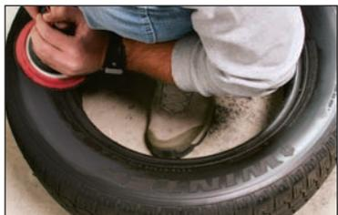
After removing the lettering, we buffed the sidewalls with 400-grit sandpaper to ensure they were smooth all the way around.
