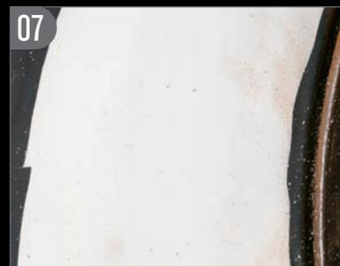
After removing the thin layer of black rubber, we noticed manufacturing imperfections around the edges of the whitewall. While these are visible up close, they are hard to see from a distance.
