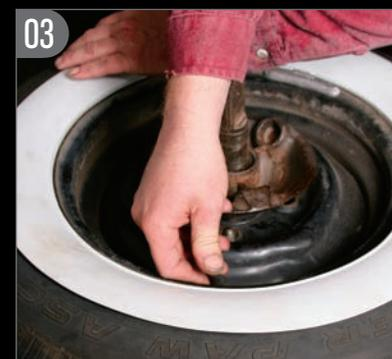
With the Port-A-Wall installed correctly and laying flat against the sidewall, we re-inflated the tire to the appropriate pressure.
