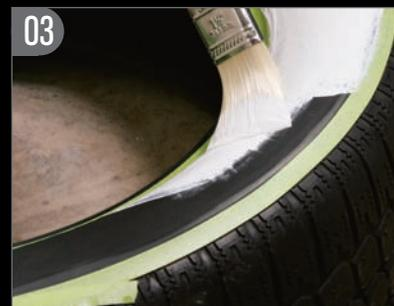
Using a brush, we applied a moderate amount of the whitewall paint to the taped off area.
