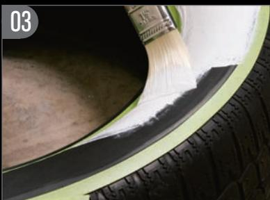
Using a brush, we applied a moderate amount of the whitewall paint to the taped off area.
