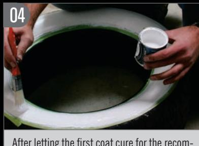
After letting the first coat cure for the recommended 24 hours, we applied a second and third coat in 24-hour increments as the manufacturer suggested.
