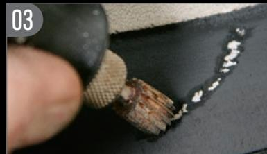
To determine the width of the tire's white rubber ring, we used a small rotary grinder to remove some of the black rubber.
