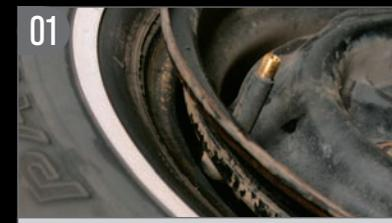
To make sure our Port-A-Walls seated properly, we separated the bead of the tire from the wheel and cleaned the mounting surfaces.
