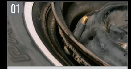
To make sure our Port-A-Walls seated properly, we separated the bead of the tire from the wheel and cleaned the mounting surfaces.
