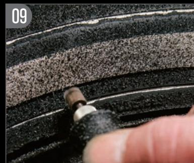
To compensate for the manufacturer's imperfections, we set our radius tool so that the rotary grinder would be approximately 1/8-inch inside the previously determined edges (step 4) of the whitewall. We then lightly scribed lines around the tire before grinding off the remaining black rubber.
