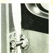
The pivoting door locks form a special feature. Although it is easy to open from inside and out, this safety lock prevents the door from flying open unintentionally or unforeseen in any situation.
