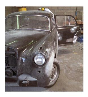
These pictures were taken during the exterior restoration. The work included body repairs, grill refinishing, painting and clearcoat. The color is dark green, as close to the original DB259, (non-metallic) Forest Green as we could get, using the chips available. Paint was done in Ditzler Durethane, by Rainbow Painting in San Luis Obispo, CA.
