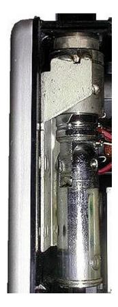
This picture shows the antenna-mount (A) of a Grundig Satellit 2000. Observe the flatter and more solid looking mount.
