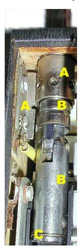
This picture shows the mount of the antenna (A) and how it fastens to the chassis. The 12-segment Grundig Satellit 205 telescopic antenna (B) has the same base diameter as the later 13-segment Grundig Satellit antennas.
