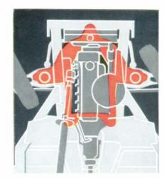
The Mercedes-Benz recirculating ball-type steering responds smoothly and precisely. A steering shock absorber protects it from road shocks.
