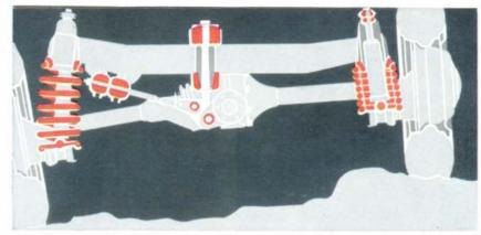
The "Sub-frame" comprehends the engine, steering and front wheel suspension in one integral unit. It insulates vibrations, regardless of whether they originate from the engine or the road, and is easily wheeled out for servicing work.
